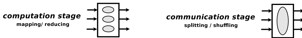
Figure 2. MapReduce Stages - Computation and Communication
