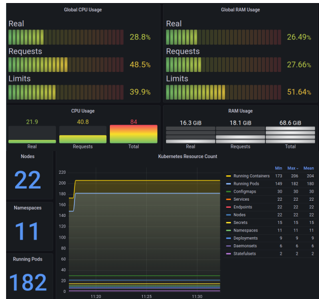
Fig. 3. Global CPU usage, global Memory usage, and Kubernetes Resource count - Grafana graph showing cluster utilization over time.
