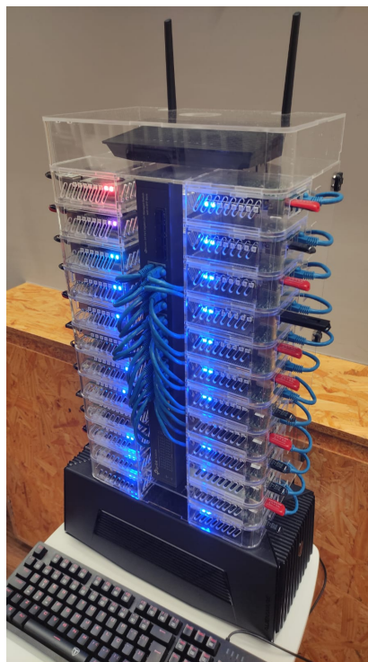
Fig. 1. UP Cluster at Insper. shows the operational Up cluster in the networking and HPC laboratory. Documentation available at https://insper.github.io/UpCluster/
