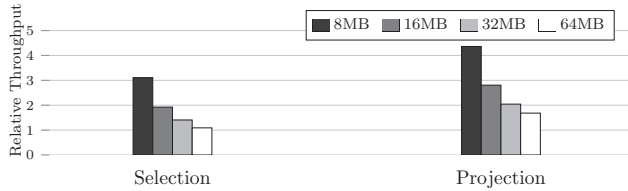
Fig. 7. Data throughput results of x86 system and VIMA executing selection and projection database queries, normalized to 16-thread x86 baseline.
