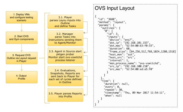
Figure 5. Open vSwitch Benchmarking Methodology
