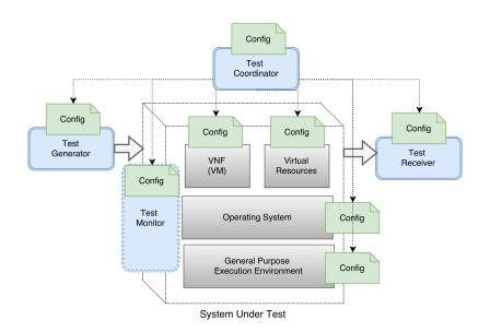
Figure 1. Big picture of VNF Testing
