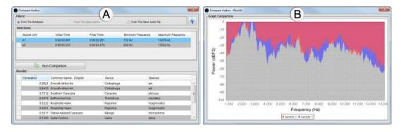
Figure 5. (A) shows the screen for audio comparison with its results, while (B) shows the data of the scientist segment (magenta) against the data of a sample from the *Descriptors* repository (blue).
