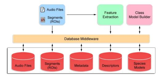
Figure 2. Structure of the data repositories.
