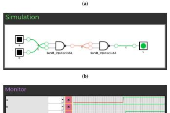
(c) **Fig. 5:** Simulation and monitoring example of the AND block shown on figure 4
